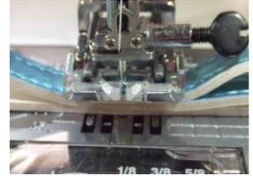
※Starting sewing...sew after the needle pierces the strap. Stitch length is 2.6
