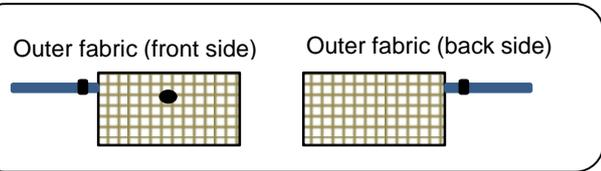
② In the middle of the lining insert ①. Sew the bag's mouth, leaving an opening ※Seam allowance 1cm
