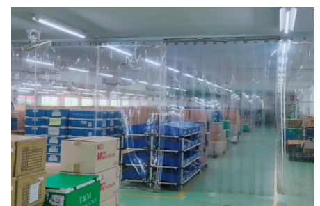
Factory partitioned by plastic curtain ( Janome Thailand Co., Ltd )
