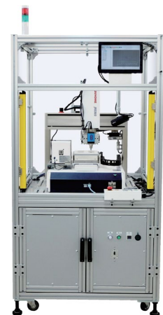
Automated Screw Tightening Robot system actually installed
