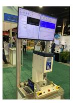
JPT0505 Servo Press with barcode reader for tracking work serial numbers
