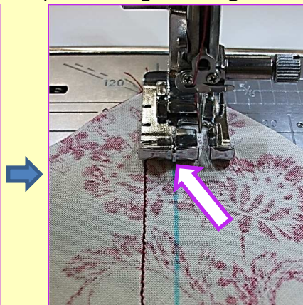
Match the 1/4" guide line with the mark and sew. As the guide line is raised, it is easy to align with the mark.
