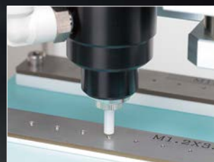
Tightens screws as small as M1.0.
